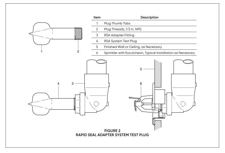
**Step 2.** Orient the sprinkler as needed by applying the manufacturer specified sprinkler wrench to the sprinkler wrench flats and tighten up to an additional full turn, or by applying up to a maximum torque of 7 lb-ft (9,5 N·m).
