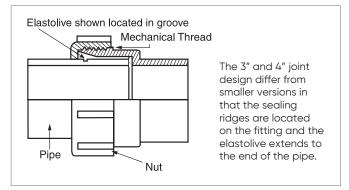
5. Place the nut onto the pipe with the threaded side to the spigot end of the pipe. Take the elastolive, stretch it and pull it over the pipe with the thick edge first and the taper pointing to the spigot end of the pipe. Slide it down the pipe and onto the groove. Once on the groove "work it" a bit to make sure that the rib on the underside of the elastolive engages the full circumference of the groove.
