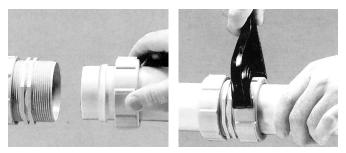
Hand-tighten the nut, then tighten, 1/4 to 1/2 turn using a spanner wrench.
