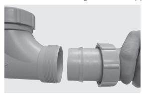
\*If you are working on a job that has the old translucent non-elastic olives, consult your "heat olive" Technical Bulletin or call IPEX Customer Services for technical information.  Apply IPEX Acid Waste Lubricant or IPEX approved petroleum jelly to both the thread and the elastolive then push the pipe squarely into the fitting.
