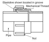
The 3" and 4" joint design differ from smaller versions in that the sealing ridges are located on the fitting and the elastolive extends to the end of the pipe.
