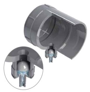
The System 636 Cleanout Condensate Drain is designed to be installed at the end of the exhaust manifold to effectively allow any accumulation of condensate or rain to drain. The Cleanout Condensate Drain is available in sizes ranging from 6" to 12" in both PVC and CPVC.
