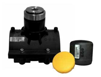
FRIALEN SPA Shut Off Saddles are the best option for areas where temporary shut off equipment may be used. The branch is threaded internally and comes equipped with a heavy brass threaded plug with gas tight O-Ring. External cap with O-Ring is used to protect Brass Plug from direct burial.
