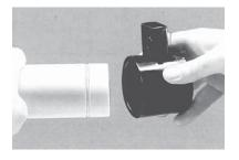
3. Examine the grooving tool to ensure that the cutting blade is fully retracted. Insert the pipe into the grooving tool.
