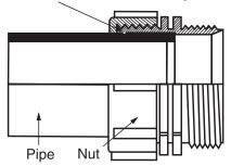
Once engaged in the groove, the elastolive virtually becomes part of the pipe and when the nut is tightened, the pipe is locked into the fitting.
