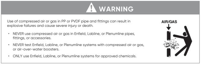
The purpose of a site pressure test is to establish that all joints have been correctly made.
