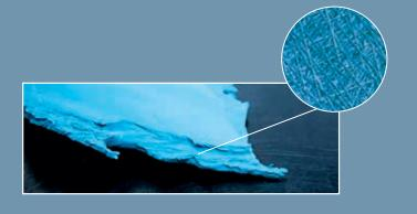
As the PVC is stretched, so are the spherical molecules, allowing more of these elongated molecules to fit into a single layer than regular PVC. This gives the material a higher molecular density and makes it tougher.
