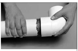
After assembly, a joint should have a ring or bead of cement completely around the juncture of the pipe and fitting. If voids in this ring are present, sufficient cement was not applied and the joint may be defective.
