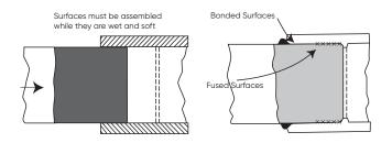
As the solvent dissipates, the solvent cement layer and the dissolved surfaces will dry and harden with a corresponding increase in joint strength. Completed joints must not be disturbed until they have properly set. See the Joint Set Schedule table for details.
