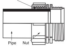
Once engaged in the groove, the elastolive virtually becomes part of the pipe and when the nut is tightened, the pipe is locked into the fitting.
