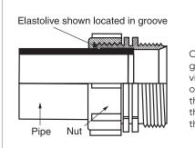
Once engaged in the groove, the elastolive virtually becomes part of the pipe and when the nut is tightened, the pipe is locked into the fitting.
