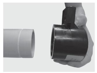
Feathered or rounded edges may indicate a worn tool and possible leakage. Make sure the groove shoulders are sharp.
