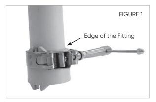
**NOTE:** The clamp should be positioned flush with the edge of the fitting. The clamp must be tightened sufficiently to prevent the pipe from rotating inside the fitting. Wheel handle clamps should not be used.
