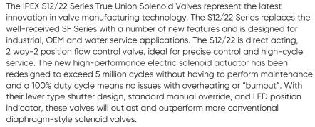
S12/22 Solenoid Valves are part of our complete system of IPEX pipe, valves and fittings, engineered and manufactured to our strict quality, performance and dimensional standards.
