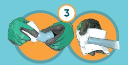
**CLEANING.** Using a clean, dry cloth, wipe any dirt and moisture from the fitting socket and the pipe end.
