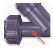
FLOW INDICATOR – The molded flow direction indicator on the side of the body ensures that the valve is installed in the proper direction.
