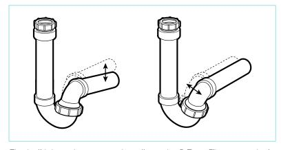
The ball joint union connection allows the P Trap Elbow to swivel up to 10° from vertical, in any direction, except directly backwards.
