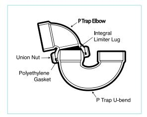
An integral limiter lug prevents the P Trap Elbow from pitching backwards providing the correct outlet slope for drainage. The polyethylene gasket ensures a leak proof connection in almost any installation situation.
