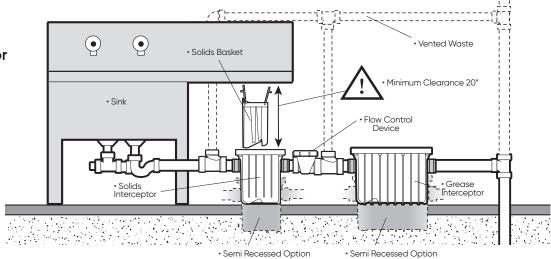
NOTE: Solids Interceptor must be installed before flow control device.
