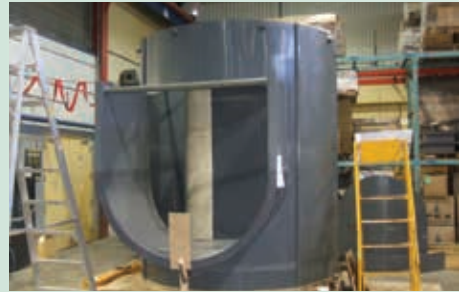
Fabrication of a 60 MGD Vortex unit Austin, Texas.
