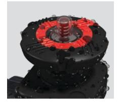
The handwheel and bonnet are made with glass-filled polypropylene (GFPP), which provides high mechanical strength and corrosion resistance. The manual handwheel and bonnet are totally waterproof, which means that all internal metal components are isolated from the external environment.
