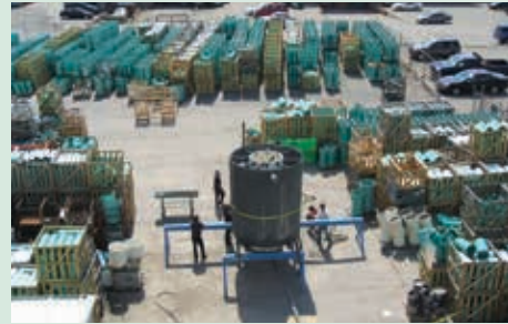
Hydrostatic testing of a large Vortex unit.
