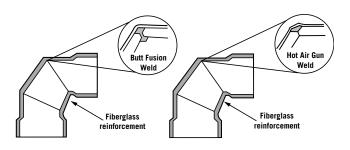
Butt Fusion Fabricated Fitting
